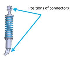
7. When the glue is still operational install the shock absorber into the model. Put bottom connector in the first step and then position the top section. If needed extend and fix the spring with water based glue (Micro Crystal Clear or Tamiya Craft Bond).
