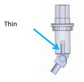
4. Put small amount of water based glue like Micro Crystal Clear or Tamiya Craft Bond into the top hole of the bottom of the shock absorber.
